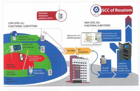
In the case of the individually set threshold values being exceeded an alarm is triggered. All data are collected, processed, visualised, archived and fed into a emergency planning forecast model for decision makers. This involves various levels of regional and national administration, including the municipality of Zelenogorsk, the region of Krasnoyarsk and the Rosatom headquarters, Moscow.
