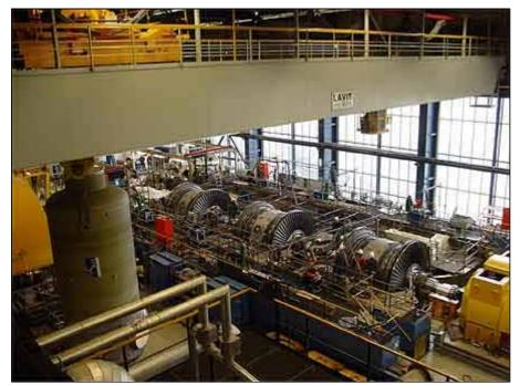
Machinefloor: inner parts of 3 LP turbines, in crane hook: new waterseparator
