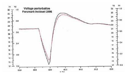
The main generator's low frequency protection was installed with erroneous phase order and therefore did not disconnect the 20 kV generator breakers in time. That disconnection would have connected in
