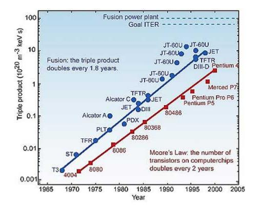
Figure 1:The progress of fusion research through the years, measured by the triple product, which is an indication of the performance of a fusion plasma. Please note the logarithmic scale on the vertical axis. F or comparison, the development of computer chips is indicated. (Courtesy of EFDA)
