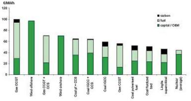
Figure 2. Indicative electricity generation new entry costs for different fuels
