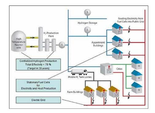
Fig. 1 Concept of a Demonstration Project for replacing fossil fuel by hydrogen and fuel cells to heat private and public houses (source Nuclear News, September 2001)
