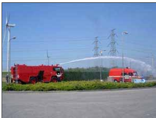
Figure 4. Crashtender for fighting kerosene fires.
