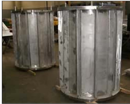
Shielded containers for activated Headstock MTR
