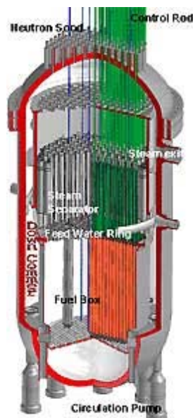
Figure 1. The High Pressure Boiling Water Reactor
