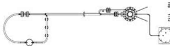
Fig. 12: MeLiLo schematics with cold trap and flange test section on left and pump with drain tank on right
