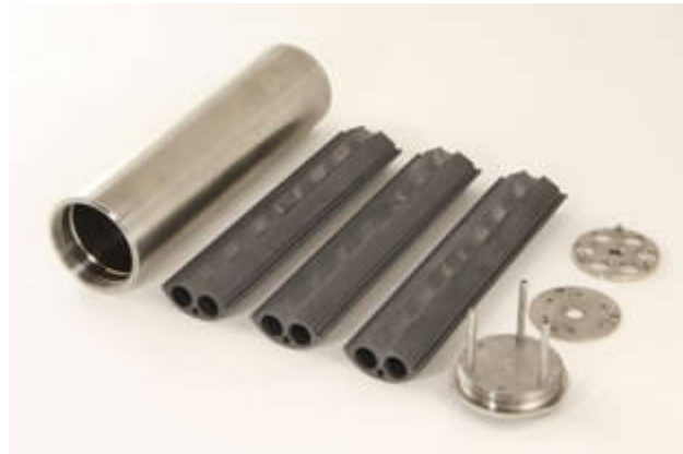
Fig. 1. Components of the experiment capsule prior to assembly. Left-to-right are the outer nickel capsule, the three sections of the graphite sample and flibe holder, and, top-to-bottom on the right, the bottom graphite support/spacer, the top cover plate, and the capsule lid (without thermocouples and gas lines).
