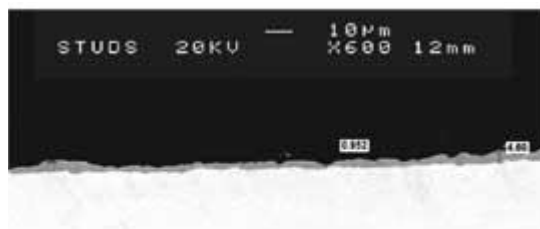
Figure 9a. 1-cycle channel. Inner surface oxide 460 mm elevation, CB-side.
