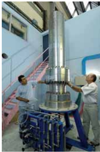
Figure 4: HETIMO test bench, thermal barrier testing, CEA Cadarache (France)
