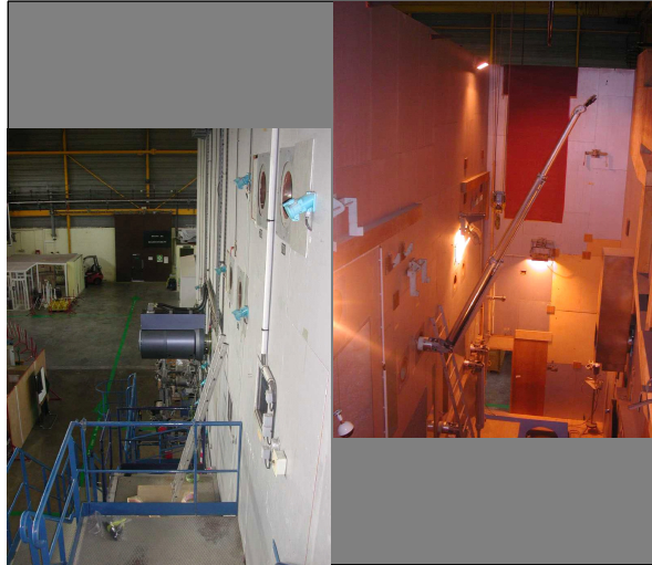
Fig. 2 –MT 200 TAO at AREVA/NC La Hague’s training and evaluation cold-cell
