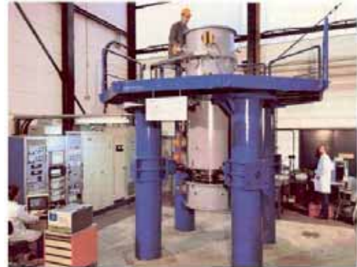
Figure 5: FLP 500, facility for testing the dynamics of a shaft supported by magnetic bearings, IPM Zittau (Germany)
