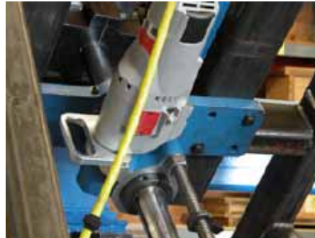
Figure 1: The boring machine with 115V variable electric drive and variable feed with special fixturing for mounting to the bottom of a steam generator.
