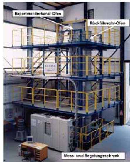
Figure 6: The NACOK air ingress integral loop, FZJ
