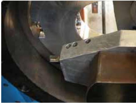
Figure 2: The boring machine with special I.D. mounting chuck and tool head for accurately positioning the cutting tool for boring a round hole to make it obround.
