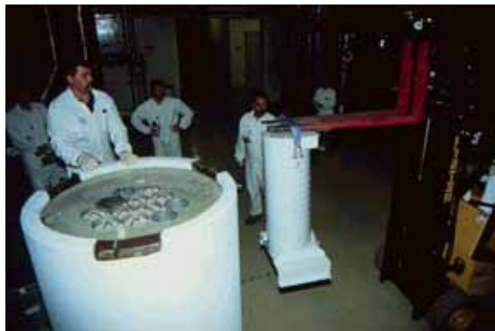
Figure 2. The final disposal container for spent ion exchange columns.
