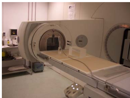
Figure 2. View of the Elekta linac upper head for 6 MeV X-ray beams and the water phantom.
