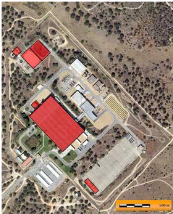
Fig. 3. Map of the Juzbado Plant showing the areas where contamination may be found (red spots)
