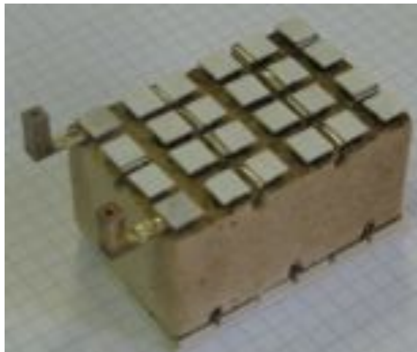
Innovative Mg-Si / Mn-Si-Ge thermoelectric module by Ecole des Mines de Nancy
