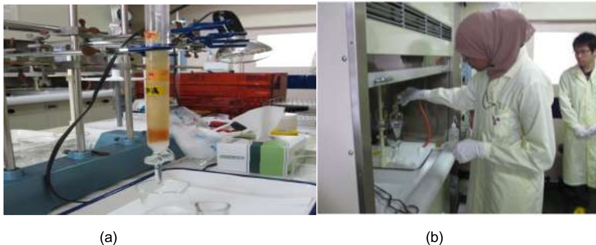
Fig. 4: (a) Experimental Apparatus of a resin column for ion exchange methods, (b) Performing the washing phase with HCl of the solvent extraction in a fume hood
