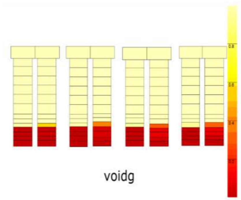
Figure 16 – Snapshot of vapor void fraction fluid temperature in the core view.
