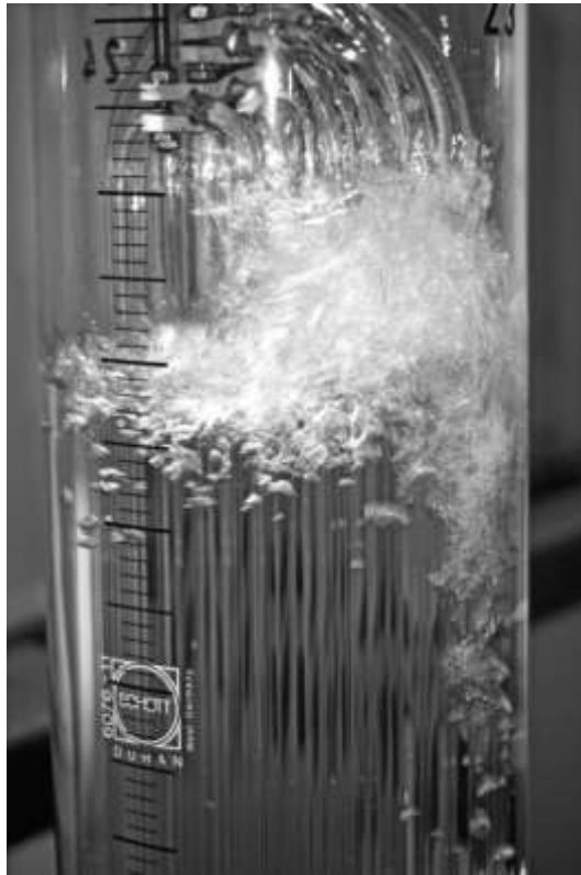
Figure 5: A steam generator during secondary side depressurization (SSD)
