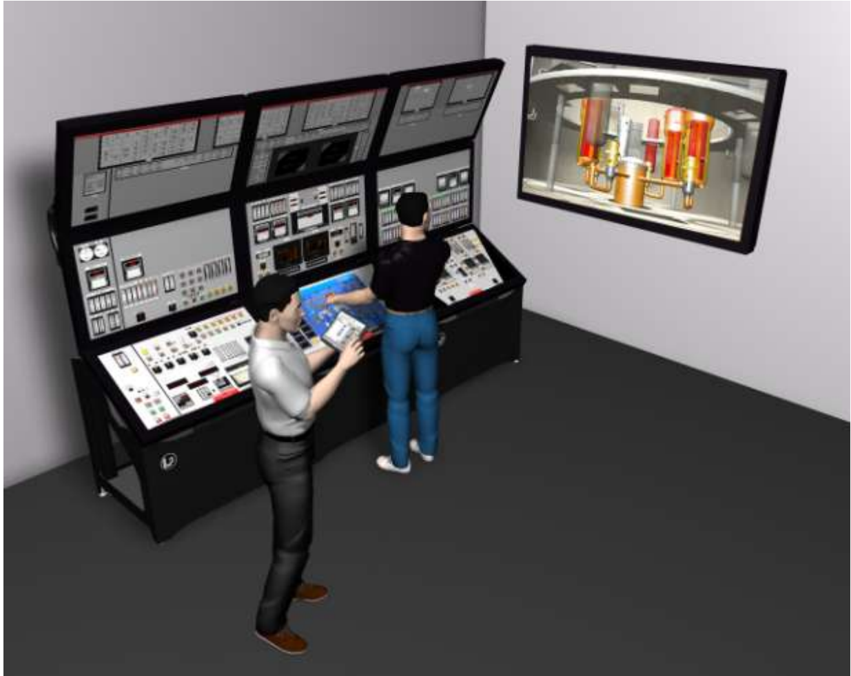
Figure 8: 3D Visualization Used in a Glasstop Simulation Environment for Operator Training
