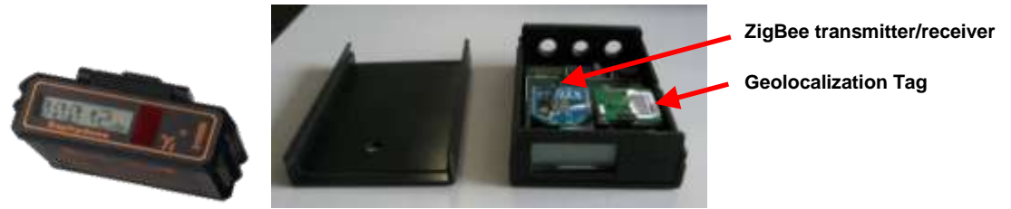
Figure 3 – Saphydose Gamma i : Real device (left) and prototype of simulation device (right)
