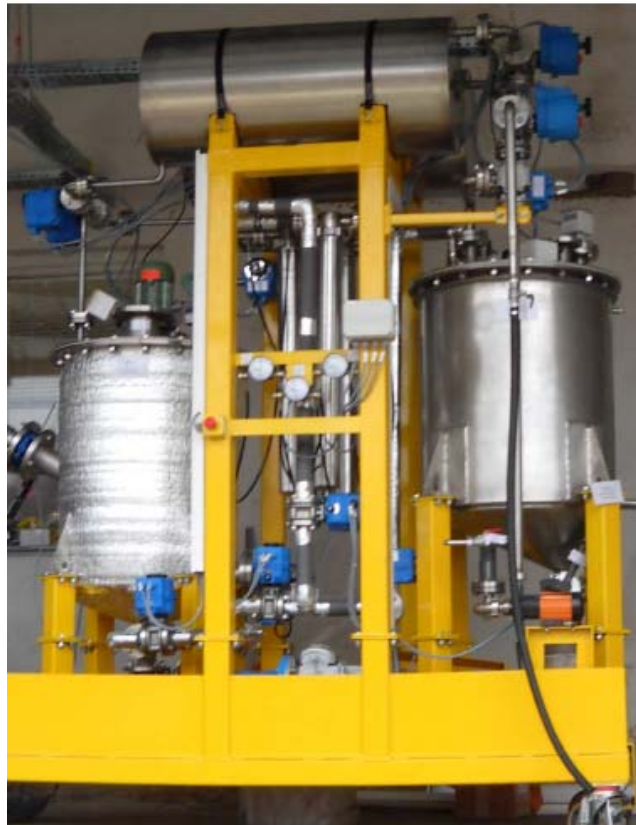
Fig.5: Pilot scale system for borate extraction.
