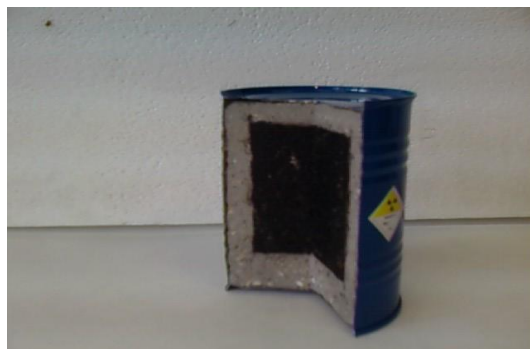
Fig 4. 200l package with conditioned resin waste
