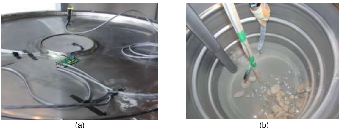
Figure 1. (a) ICT fitted to underside of waste container lid (b) waste container with sensor harness being filled with reference grout
