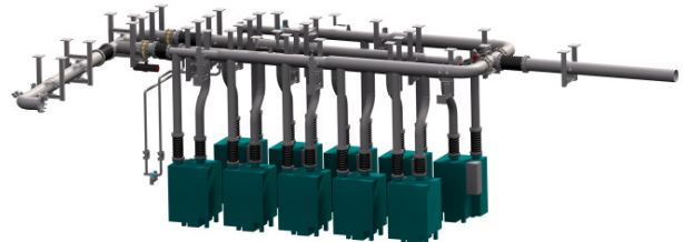
Fig. 5: HEPA filter rack
