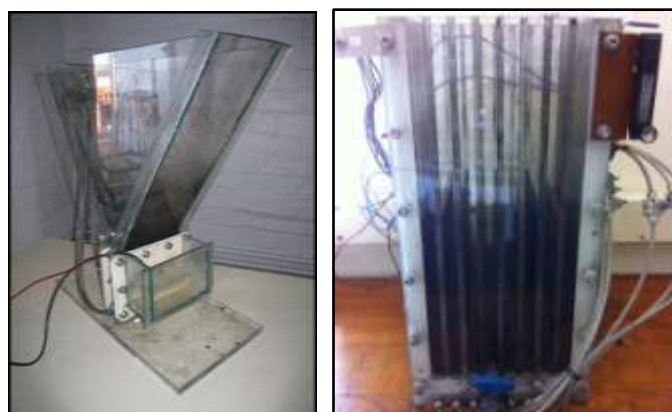
Fig 2. – Laboratory scale batch reactors (1-cellsystem (L) 4-cell System)
