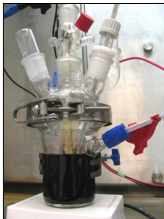
Figure 1. (left) Lab scale \text{PuO}_2 dissolver; (right) A typical [\text{Pu}] vs time plot (final [\text{Pu}] = 100\text{g/l} )
