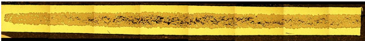
Fig 6. Optical micrographs showing the development of voids, leading to excessive swelling as observed in the FUTURE U(Mo)-Al dispersion fuel plates.
