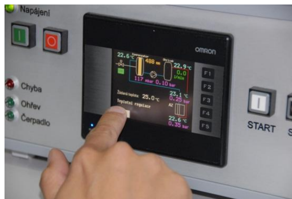
Fig. 4 Touch-screen of the instrumentation control unit
