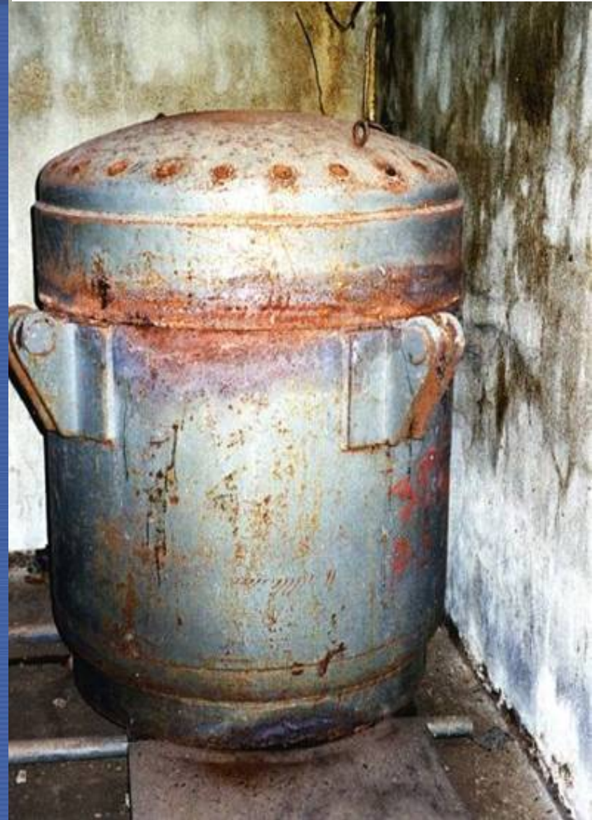
DISUSED TELETHERAPY HEAD IN TRANSPORT CONTAINER Cs-137 ~ 26 TBq (700 Ci)
