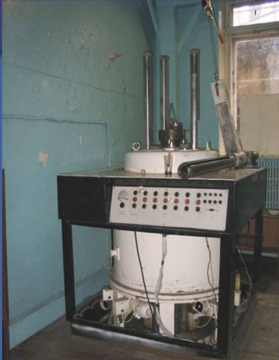
DISUSED SELF-CONTAINED IRRADIATOR Co-60 ~ 370-740 TBq (10-20,000 Ci)
