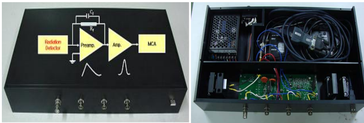
Fig. 3. Prototype of the spectroscopy system with the lid open and closed
