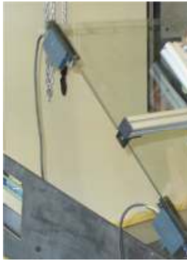
Fig 4 - Haptic actuators on the tactile slab
