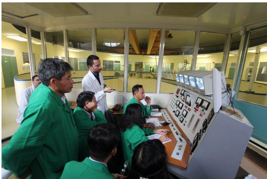
Fig. 4: Reactor operation exercise at BME Training Reactor
