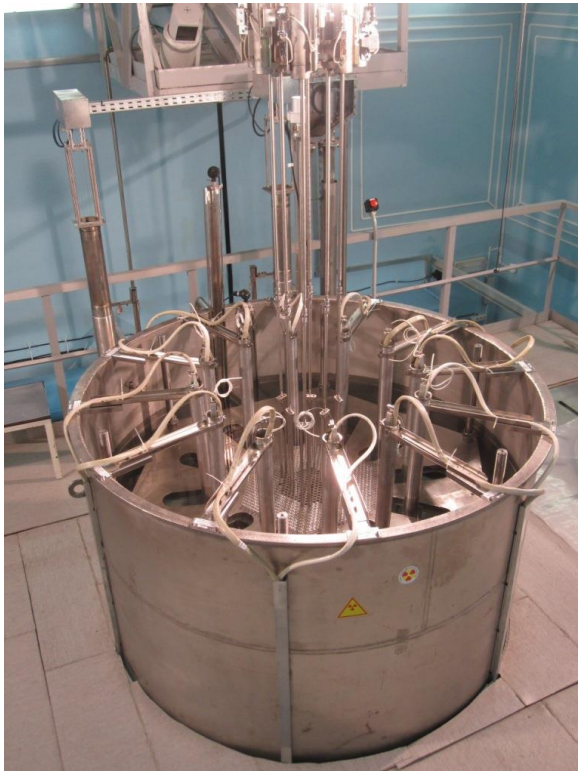
Fig 3. Critical assembly with a water moderator
