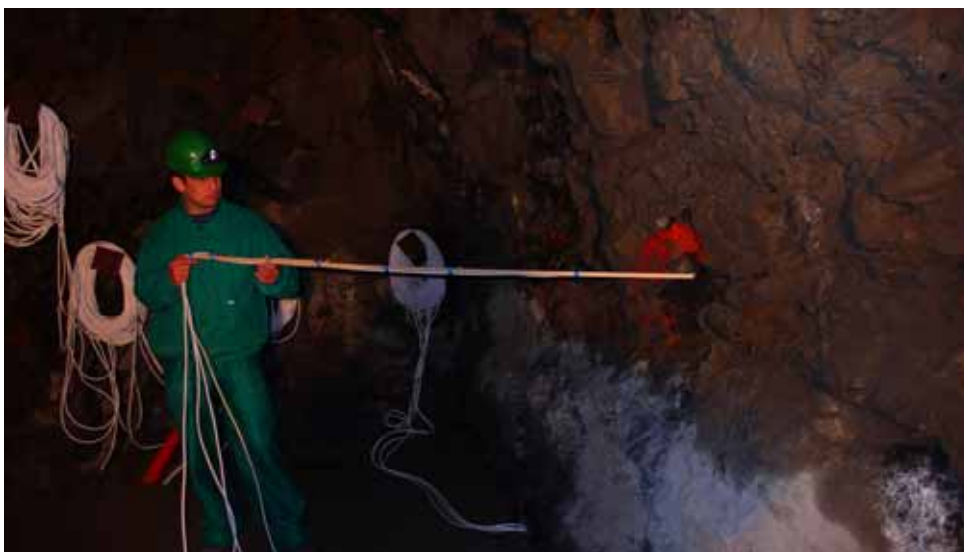
Fig. 2. Installation of thermometers
