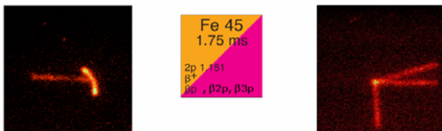
Fig 5. Camera recording of 2p and \beta 3p decay events in ^{45}\text{Fe} [11]. Left: A track of a ^{45}\text{Fe} ion entering from left. The two short tracks are protons of \sim 0.6 MeV. (image courtesy of M. Pfützner). Right: three tracks of protons following the \beta^- decay (Reprinted with permission K. Miernik, et al., Phys. Rev. C 76 , 041304 (2007). Copyright (2007) by the American Physical Society). Centre: updated nuclide information for ^{45}\text{Fe} shown in the nuclide chart.
