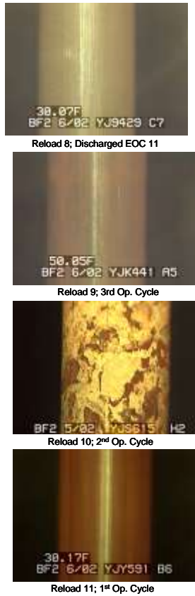
Figure 2: Visual Appearance of Fuel Rods in BF-2 Reloads 8, 9, 10 and 11
