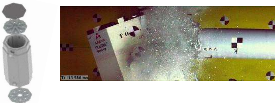
Fig 5 : TN NOVA™ dry storage system - aircraft crash test
