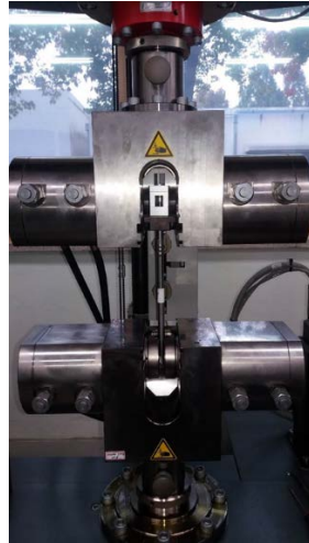
Fig. 5. Set up of the strength test of the reinforcement device
