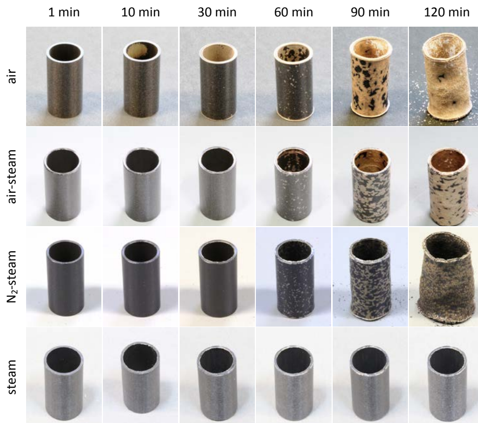
Figure 3: Post-test appearance of samples oxidised at 900°C in specified atmospheres.
