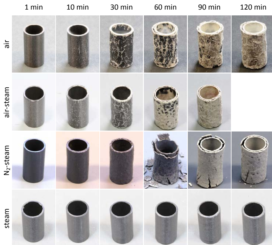
Figure 5: Post-test appearance of samples oxidised at 1100°C in specified atmospheres.
