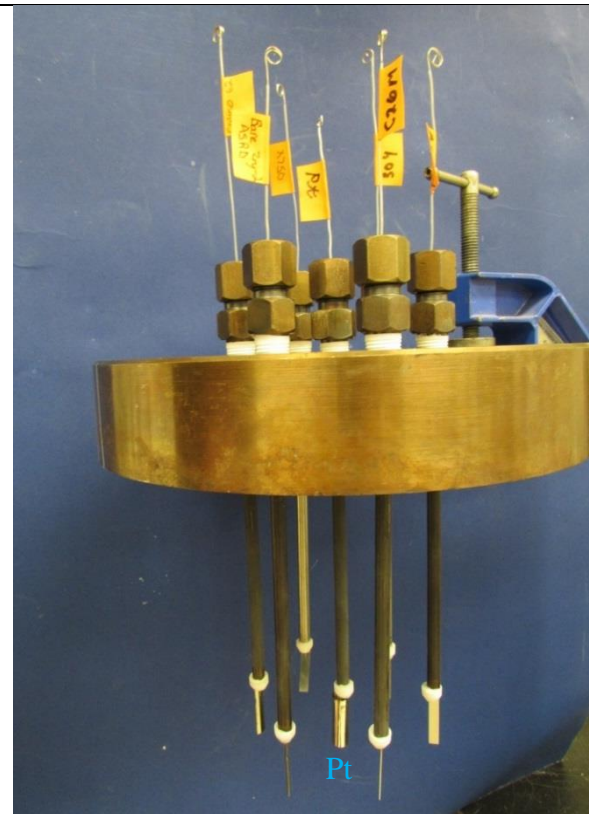
Figure 2. Six specimens mounted in the autoclave head. The Pt counter electrode is at the center
