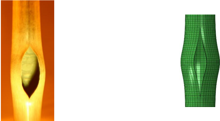
(a) Cladding tube after LOCA test [5] (b) FEM model of burst cladding tube
