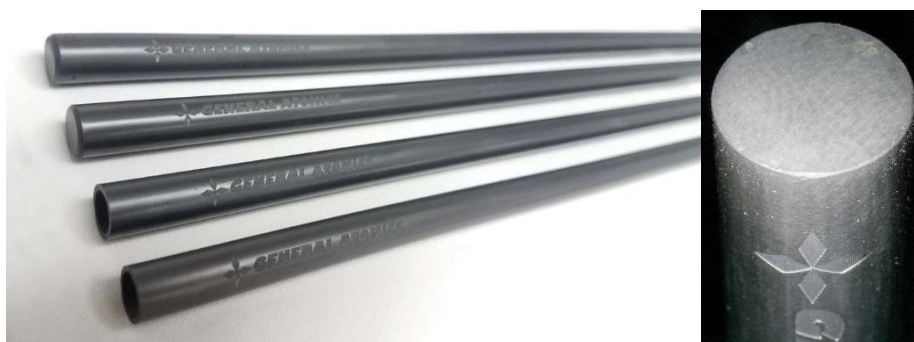
Fig. 1: (left) examples of open and closed end SiC-based cladding tubes, and (right) magnified view of SiC-cladding tube sealed with a SiC endplug and HSiC joint
