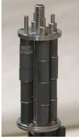
Figure 1d. Sample holder and loading in the test rig
