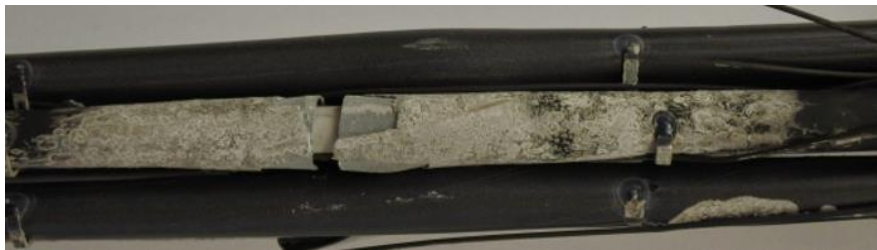
Fig. 11. View of the CODEX-LOCA-E4 bundle after the test
