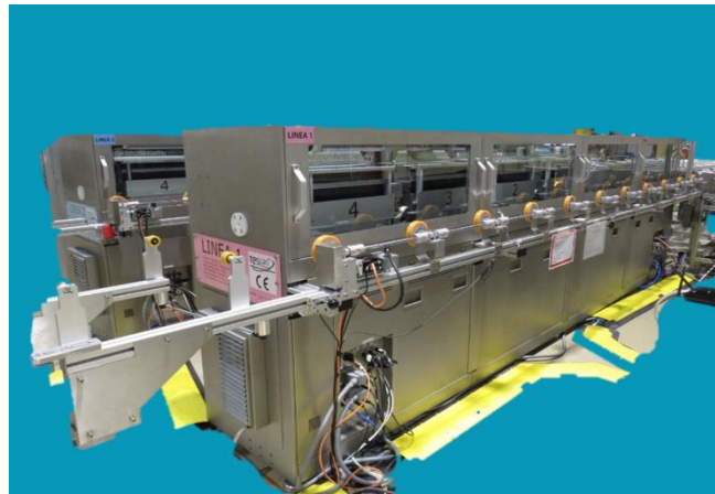
Figure 6. Passive Gamma Scanner High Speed
