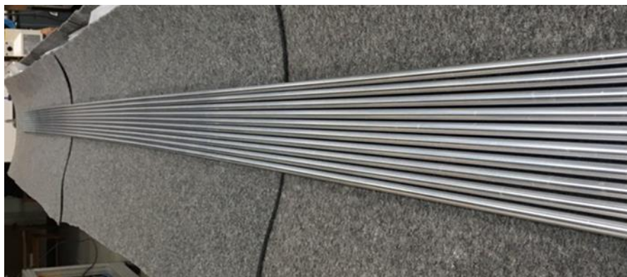
Fig 4. Example of Cr-coated full length tubes fabricated using the prototype showing uniformity of the visual aspect over the full length.
