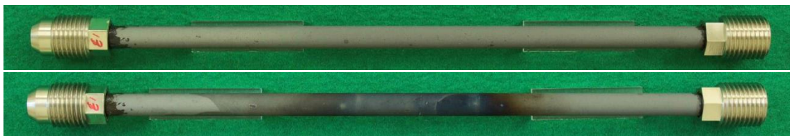
Fig 4 Visual appearance of the SiC/SiC sample tube before (upper) and after (lower) temperature elevation test. (Initial internal pressure of the tube: 7 MPa)
