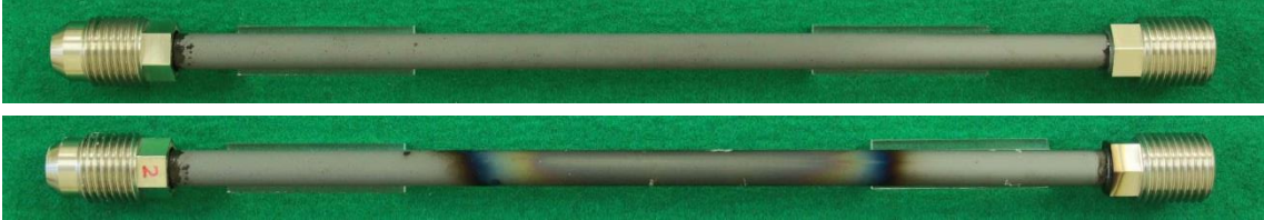
Fig 6 Visual appearance of the SiC/SiC sample tube before (upper) and after (lower) of the LOCA integral test.
