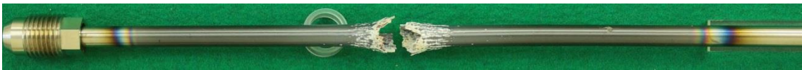
Fig 8 Visual appearance of the Zr-based alloy sample tube after the LOCA integral test.
