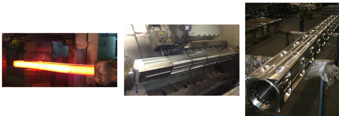
Figure 2: Manufacturing process of the PWR-Quiver base body.
