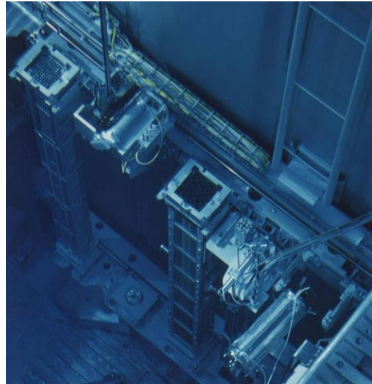
Figure 4. Coordinate Wagon driving the lower part of a fuel rod from one assembly to another in the loading pool at KKG. Right: Detail of the Coordinate Wagon between two assemblies.
