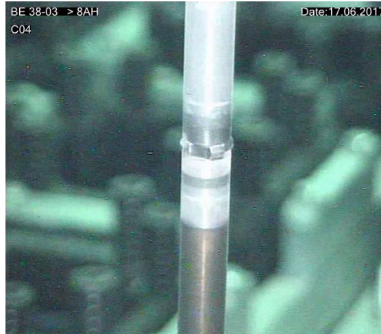
Figure 6. Visual appearance of the Cr-coated M5 lowermost segment of MTR with the denomination C04, after one cycle irradiation (maximum neutron fluence of ca. 3 \times 10^{21} n/cm 2 ). The Cr-coating is best to be seen on the colour picture (top-right).
