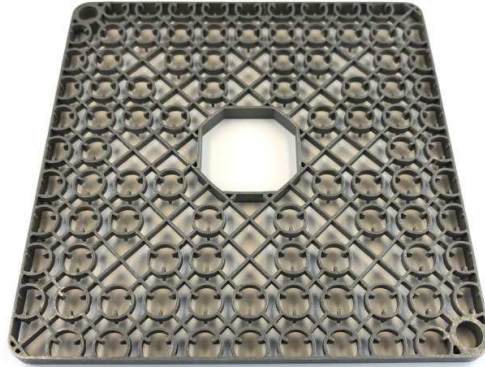
Fig 3: Grid for UTP made with AM
