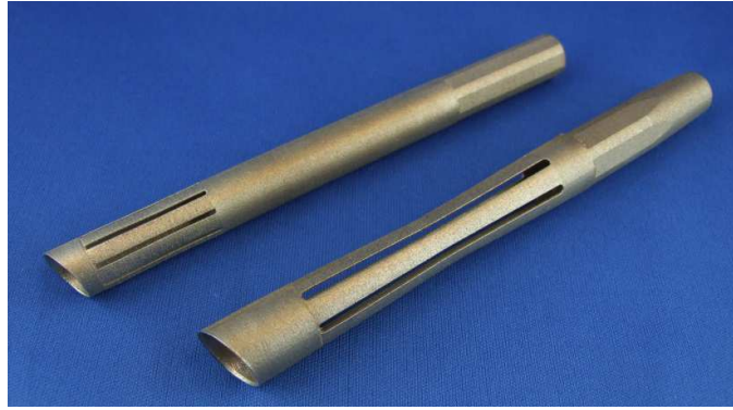
Fig 5: Tools to grab fuel rods
