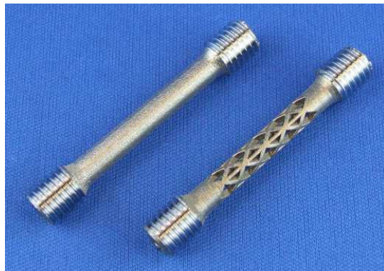
Fig 10: Samples for out of pile testing
