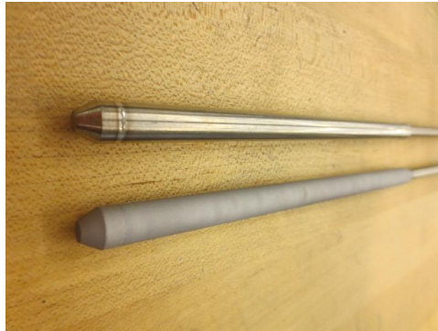
Fig. 1: Uncoated Zircaloy-4 sample (top) and Cr coated (bottom).
