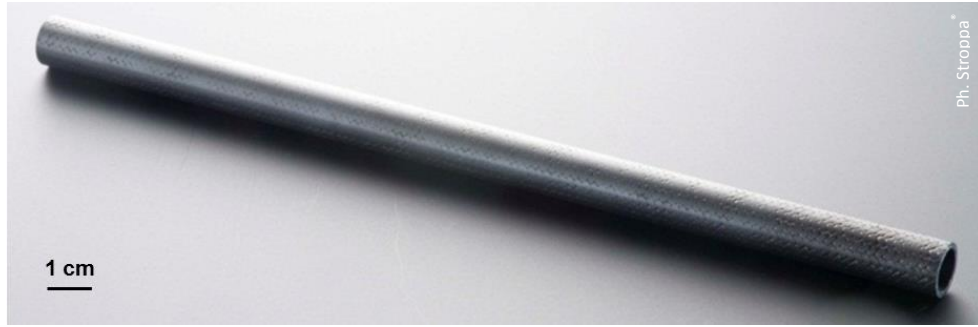
Figure 1: Representative \text{SiC}_f/\text{SiC} tubular specimen processed at CEA
