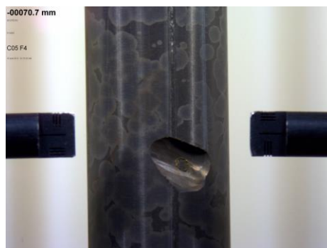
Figure 1: example of a fuel rod with a through-wall defect due to debris fretting
