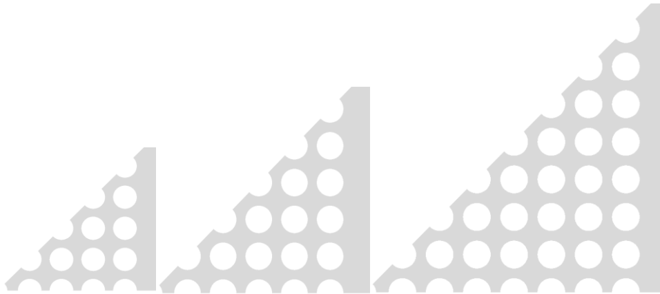
Figure 6 : geometries of the fuel rod bundles with 4, 5 and 7 rod rows around the leaking fuel rod (1/8 of the rod bundle is represented; an “absorbing” boundary condition is set on the right side of the meshing)
