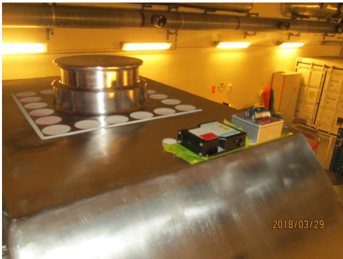
Figure 1, mounting of two different accelerometers outside the TN17 cask
