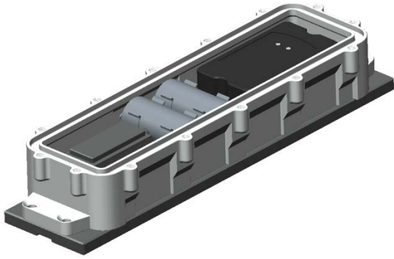
Figure 3, holding equipment for two accelerometers inside the square tube of the dummy fuel
