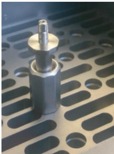
Fig. 6. ESPIGA top end on the top nozzle plate at the instrumentation tube location
