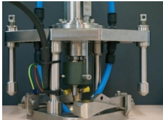
Fig. 4. Electrical discharge machining (EDM) equipment, used to drill the top nozzle plate
