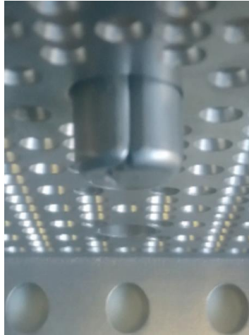
Fig. 5. ESPIGA bottom end through the bottom nozzle plate at the instrumentation tube hole
