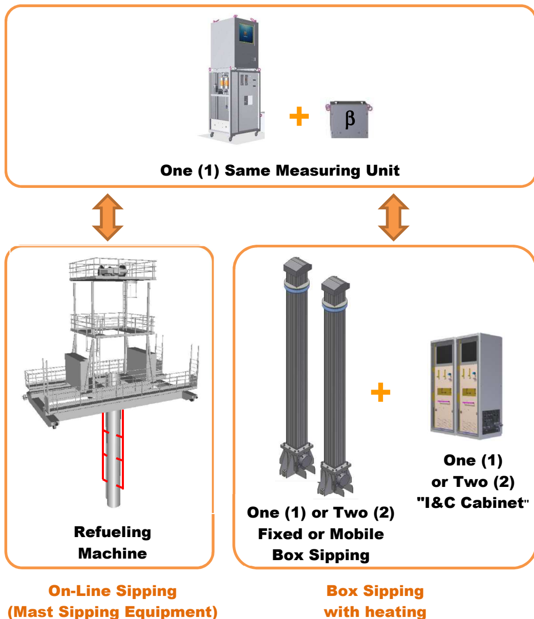
Fig 2. On-Line Sipping and Box Sipping with heating can share same measuring unit
