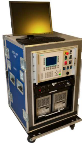
Fig 4. Framatome sipping electrical console
