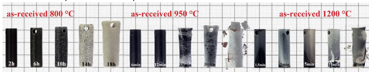
Fig. 4: Visual comparison of as-received cladding specimens of E110 alloy after high temperature oxidation in air.
