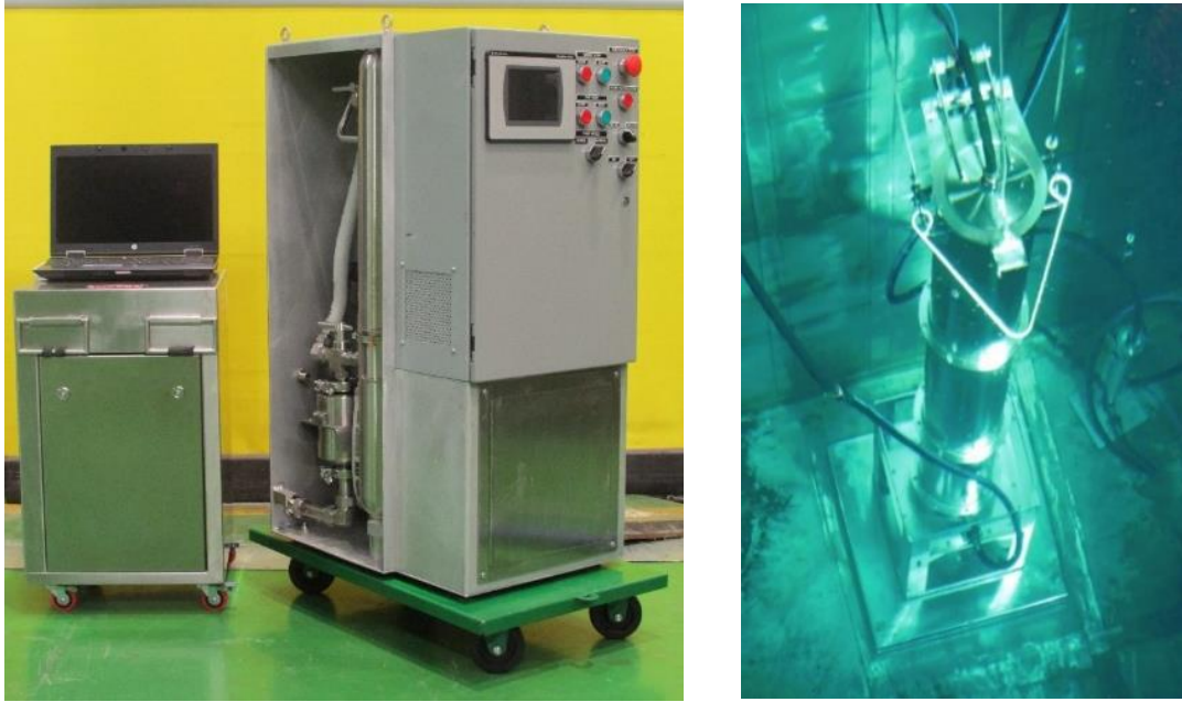
Fig 1. SICOM-INCAN SIPPING: Detection unit, Process unit and canister.
