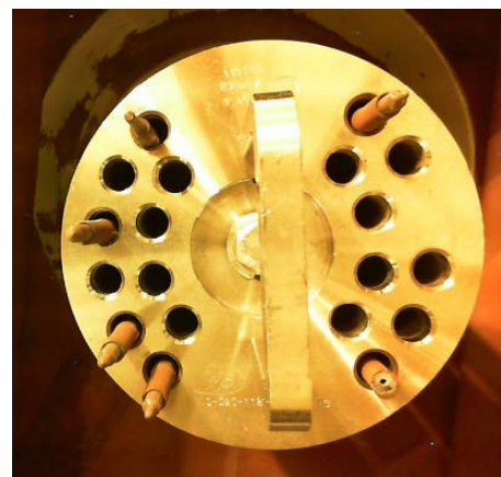
Fig 5 - The centering frame in the unloading position at the Studsvik hot cell and a front view the centering frame in the hot cell before retrieval of the rods
