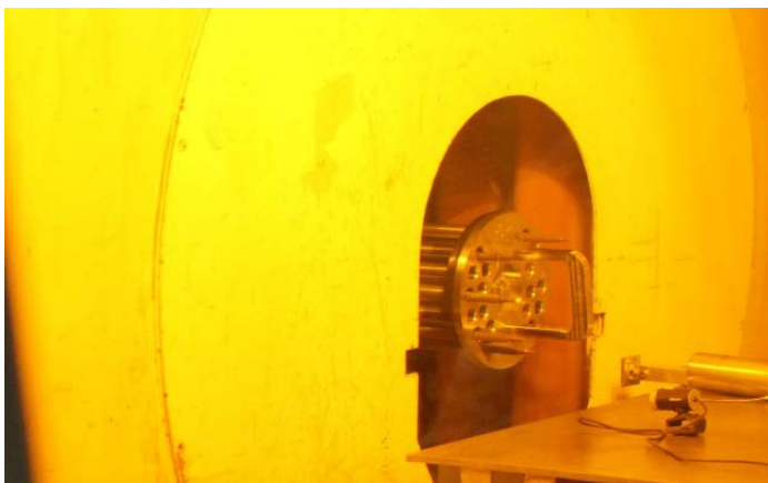
Fig 5 - The centering frame in the unloading position at the Studsvik hot cell and a front view the centering frame in the hot cell before retrieval of the rods
