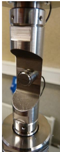
Figure 1. The ring tensile setup (Instron 8562) at the standard NRG's reference laboratory.
